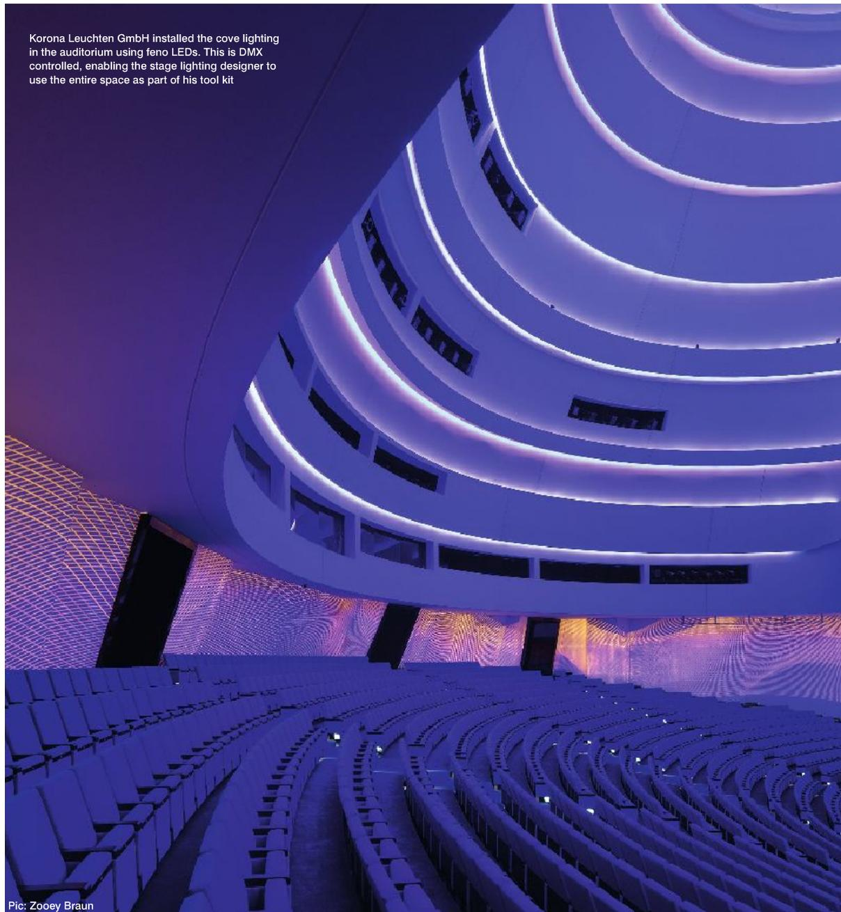
Korona Leuchten GmbH installed the cove lighting in the auditorium using feno LEDs. This is DMX controlled, enabling the stage lighting designer to use the entire space as part of his tool kit
